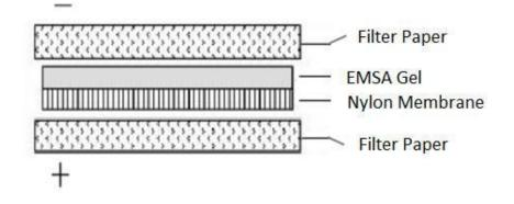
(4) Semi-dry electro-transfer: perform transfer in 0.5× TBE at constant 300mA for 20 minutes.
