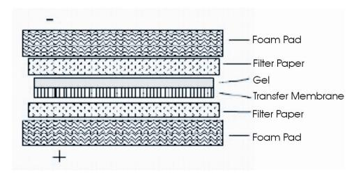
(4) Transfer: Transfer in 0.5× TBE at 390mA for 40 minutes.
